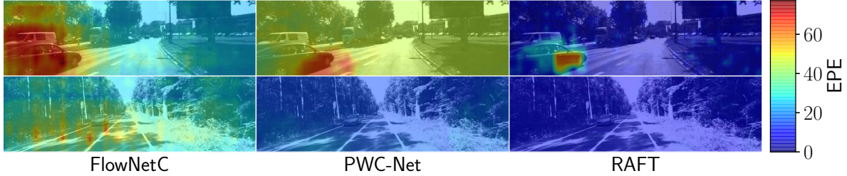
Figure 2. Impact of spatial locations. Effect of the spatial location of an adversarial 102 \times 102 patch. Best viewed in color.
